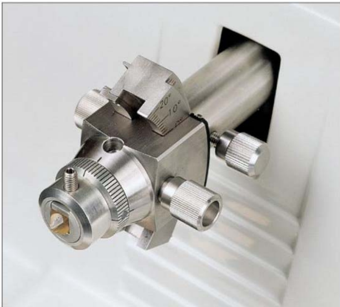
(b) Microtome arm of ultramicrotome
